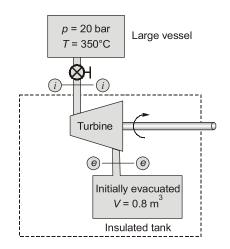
$$m_i \left( h_i + \frac{V_i^2}{2} + gz_i \right) + Q - m_e \left( h_e + \frac{V_e^2}{2} + gz_e \right) - W = (m_2 u_2 - m_1 u_1)_{\text{turbine}}$$
